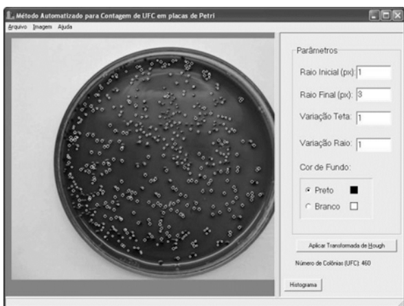
Figure 5 - The white circles show the processed image the colonies detected
