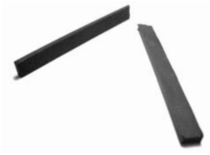
Figure 1: Samples of SiC cut in the dimensions of the guitar saddle.
