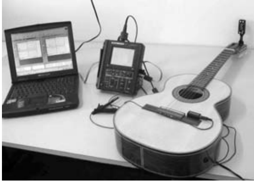
Fig.3: waves acquisition using a pickup connect with the oscilloscope Tektronix
