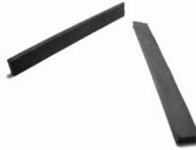
Fig. 1: Samples of SiC cut in the dimensions of the guitar saddle.
